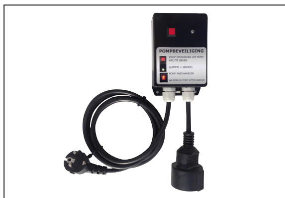
Pump safety , is mounted between the pump and socket, and releases the pump for 5 minutes. This device prevents damage to the pump that would inadvertently be caused by its continued running. Article number: PB-02
